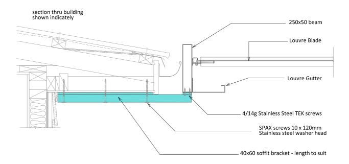
Fixing of Soffit brackets for the mounting of the louvre assembly. Initially mount only two brackets being the brackets closest to the each end of the support beam, once the beam is inplace then line up all other required brackets
