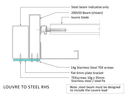
Important Note: Screw or bolt fixing centres required for the Louvre roof to any building element refer to Louvre Design Manual Sections 6.0 Bracing Requirements and 7.0 Supports use these tables to calculate maximum Tributary areas for bracing / bracket centres.
